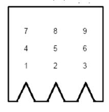
**Note:** To obtain local control using the internal potentiometer accessible at the top of the unit, jumper P2 pin 4 to pin 9.
